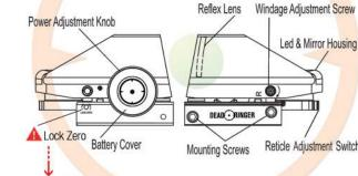
Caution: Loosen lock screw before making windage or elevation adjustments using the provided screwdriver
